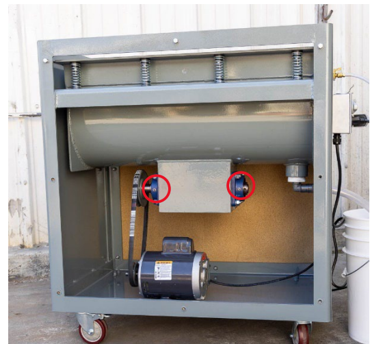
Figure 2 QDB3 Internal Configuration. Zerk locations circled in red
